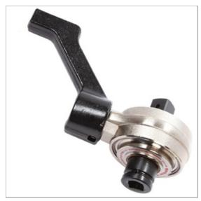
The 'Highwayman' torque multiplier has been designed for use where it is necessary to provide higher torques than would otherwise be possible due to limitations of space or operator strength. Input to the multiplier is via a ratchet torque wrench set to one fifth of the desired output torque.
