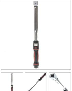
Norbar Torque Handles are based on the 'Professional' wrench range and share the same high precision engineering. The Female End versions are either  $9 \times 12$  mm or  $14 \times 18$  mm rectangular type. For many applications a spanner end fitting rather than a socket is the best or, often, the only solution. Typically this will be because the joint is a pipe union (such as a brake pipe).
