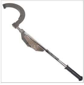
The correct tightening of carbon/graphite electrodes is known to increase the energy efficiency of electric arc furnaces and prevents electrode sections from being lost in the furnace. Norbar Electrode Wrenches are based on two well proven torque wrench designs: electrodes up to 8 inches use the 'Professional' type, 9 inches and upwards are based on the 'Industrial' wrench.
