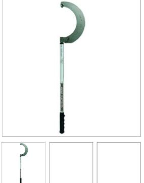
The correct tightening of carbon/graphite electrodes is known to increase the energy efficiency of electric arc furnaces and prevents electrode sections from being lost in the furnace. Norbar Electrode Wrenches are based on two well proven torque wrench designs: electrodes up to 8 inches use the 'Professional' type, 9 inches and upwards are based on the 'Industrial' wrench.
