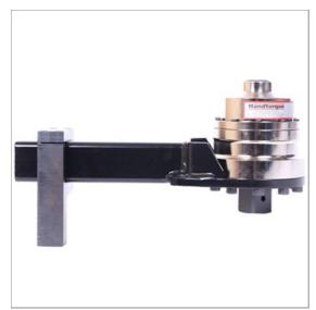
Norbar 'HandTorque' multipliers employ multiple stages of epicyclic gearing to give a wide range of torque outputs and ratios to suit most applications. Ratios quoted are always the torque multiplication ratio, not the velocity ratio as given for some competitor's products. For example, the velocity ratio may be 29.8:1 to give a torque multiplication of 25:1 ±4%.
