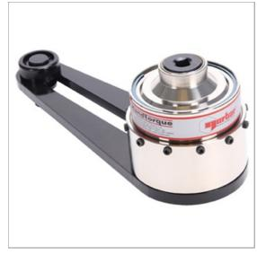
Norbar 'HandTorque' multipliers employ multiple stages of epicyclic gearing to give a wide range of torque outputs and ratios to suit most applications. Ratios quoted are always the torque multiplication ratio, not the velocity ratio as given for some competitor's products. For example, the velocity ratio may be 29.8:1 to give a torque multiplication of  $25:1 \pm 4\%$ .
