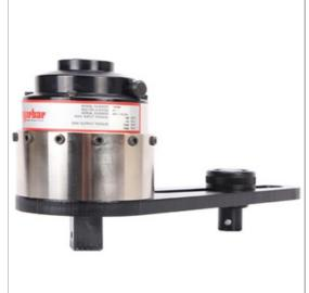
Norbar 'HandTorque' multipliers employ multiple stages of epicyclic gearing to give a wide range of torque outputs and ratios to suit most applications. Ratios quoted are always the torque multiplication ratio, not the velocity ratio as given for some competitor's products. For example, the velocity ratio may be 29.8:1 to give a torque multiplication of  $25:1 \pm 4\%$ .
