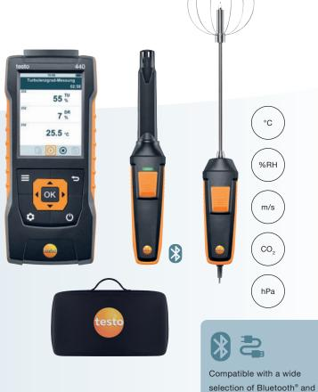
With the testo 440 comfort level ComboKit with Bluetooth®, all IAQ-related parameters can be measured and documented wirelessly. The testo 440 air velocity & IAQ measuring instrument recognizes probes automatically, and its structured measurement menus simplify the adjustment of air conditioning and ventilation systems. In addition to a Bluetooth® probe, a wired probe and a thermocouple Type K temperature probe can also be connected to the measuring instrument.
