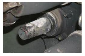
After the first pothead fuse was closed to this feedthrough three-phase transformer, it began to rattle furiously. Seconds later an uncapped bushing flashed over.
