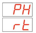
The second available mode is Real Time which displays the current as it normally rises or falls. Real Time mode allows the user to see changes in load current as they occur.
