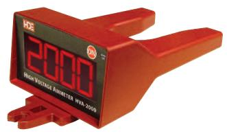
The initial factory default mode is Peak Hold, which displays the peak RMS current measured while the Ammeter is placed on a conductor. Peak Hold mode allows a user to capture and store the peak current over the period of time the Ammeter is applied to a conductor.
