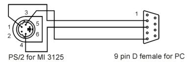
Figure 6.14: Interface connection for data transfer over PC COM port
