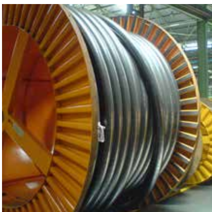
➤ Cable on drum, 115kV single core
