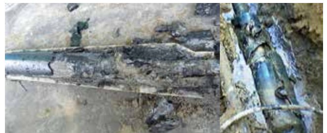
➤ vaporized core after cable fault, 132 kV XLPE
