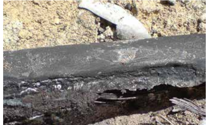
➤ vaporized core after cable fault, 132 kV XLPE
