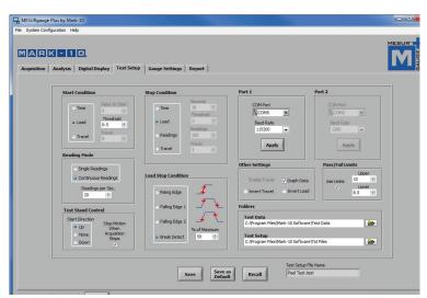
Configure test start and stop conditions.
