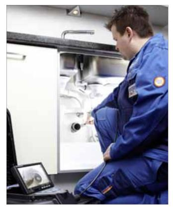
The robust color camera head is waterproof to 3 bar. With a diameter of just 26 mm it easily negotiates  $87^{\circ}$  bends in pipes of Ø 40 mm and larger.
