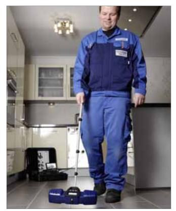
The actual meter count and the position of the head are displayed in the monitor. The Wöhler L 200 Locator makes it possible to locate the camera.
