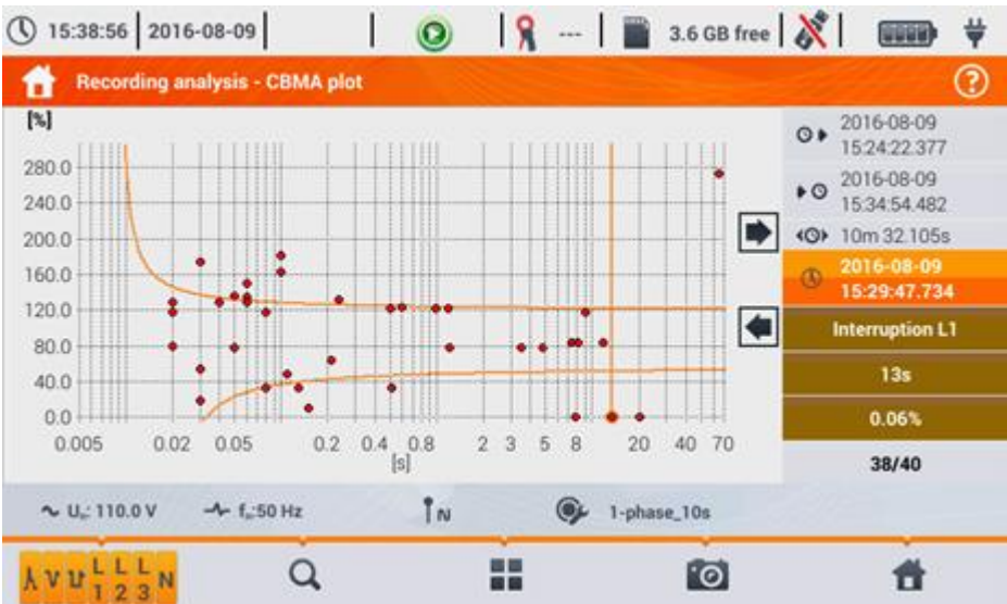
Fig. 32. Recording analysis - CBEMA graph.
