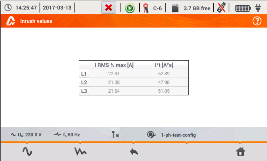
Fig. 44. Inrush current - characteristic parameters.
