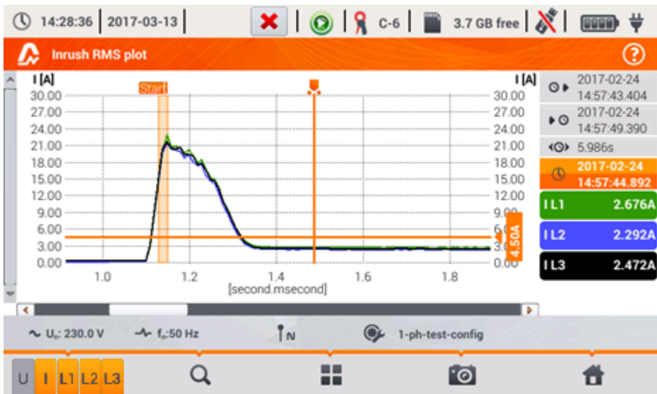
Fig. 43. Inrush current analysis – Inrush RMS plot.
